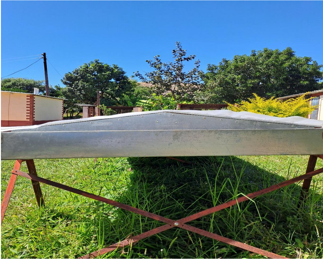
Figure 4.3 Sample of a backyard solar drier measuring 5.5 metre-long and 1.6 metre wide, one by 50 watt solar panel and one by 50 watt DC fan
