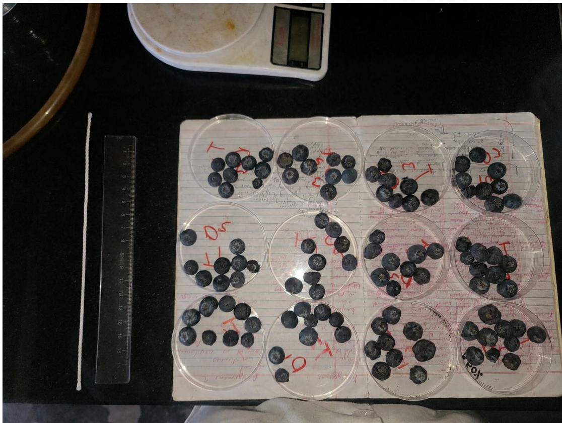
Figure C7: String and ruler used to estimate berry diameter from circumference measurements, shown alongside the Petri-dish replicates.
