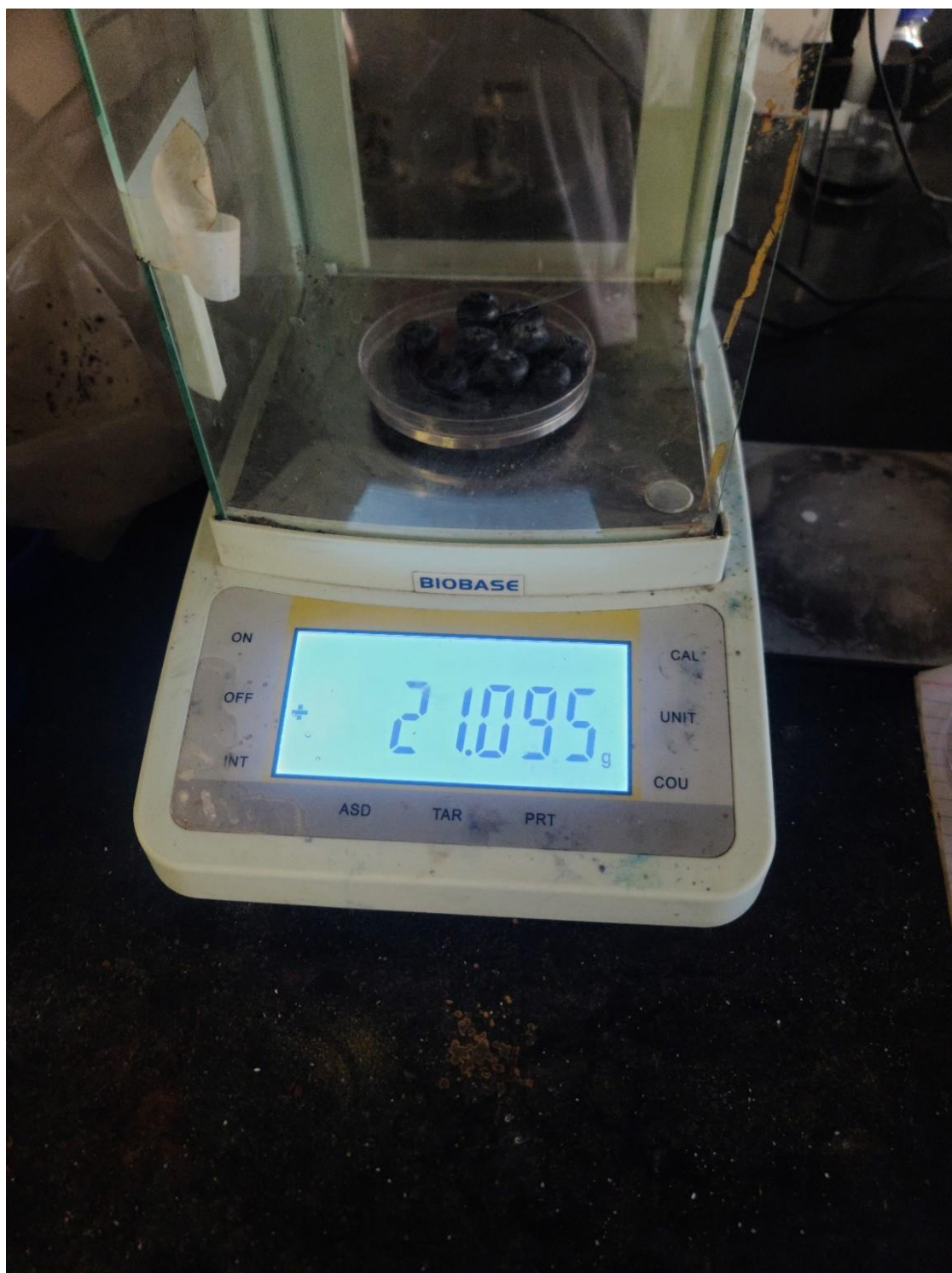
Figure C6: Representative weighing of a Petri-dish replicate on the analytical balance during the storage study.
