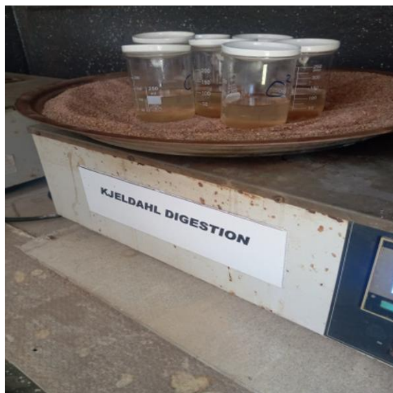
Figure 4 Kjeldahl digestion with a tray of sand
