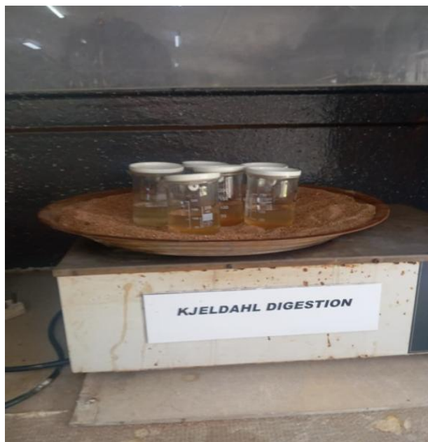
Figure 4 Kjeldahl digestion with a tray of sand
