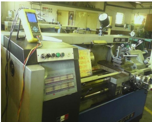
Fig. 1. Cazeneuve 360 HB-X precision lathe machine
