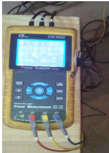
Fig. 1. Lutron 3 Phase digital Power Analyser/meter
