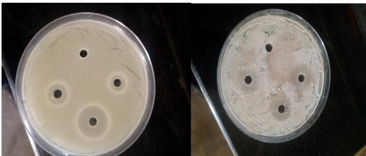
Figure 4.1: Plates showing ZOI for bacteria ( E. carotovora ) (left) and fungi ( B. cinerea ) (right)
