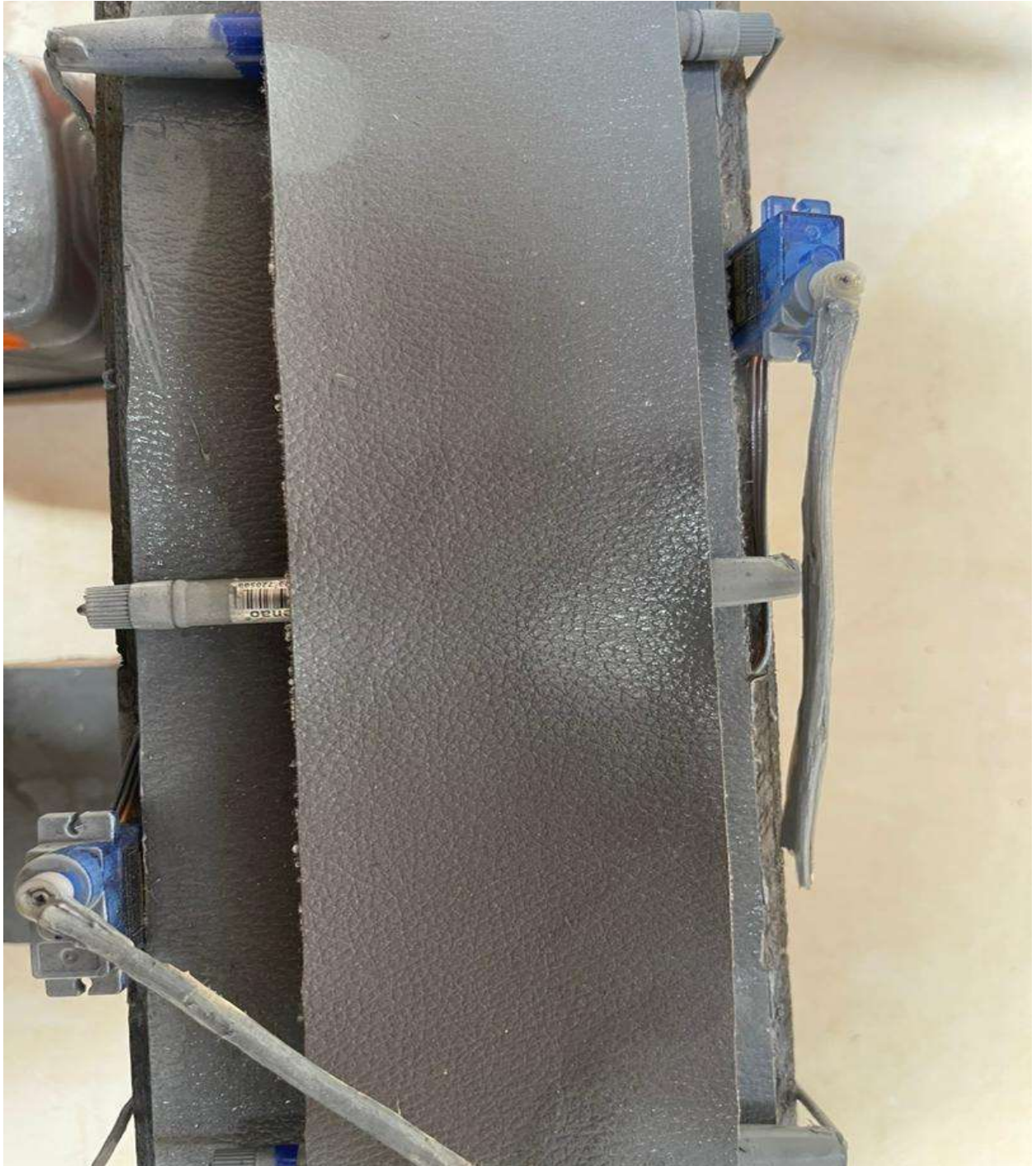
Figure 4:5 servo placement on the conveyor
